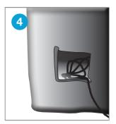
Place the pump and excess wires into the access cavity ensuring that the long pump wires extend out through the opening.
