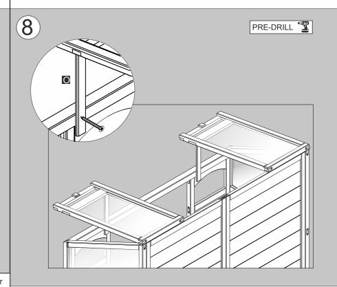
Place the prop against the inside of the front batten. Position the screw so that the prop can be turned both ways and offer two settings for ventilation. Use a single 40mm screw.
