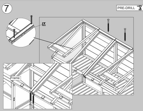
Place the two (fixed windows) on to the green house. These must be in line with the two outer opening windows. They must each be placed so that there is a small gap between these and the outside opening windows to allow them to open freely.
