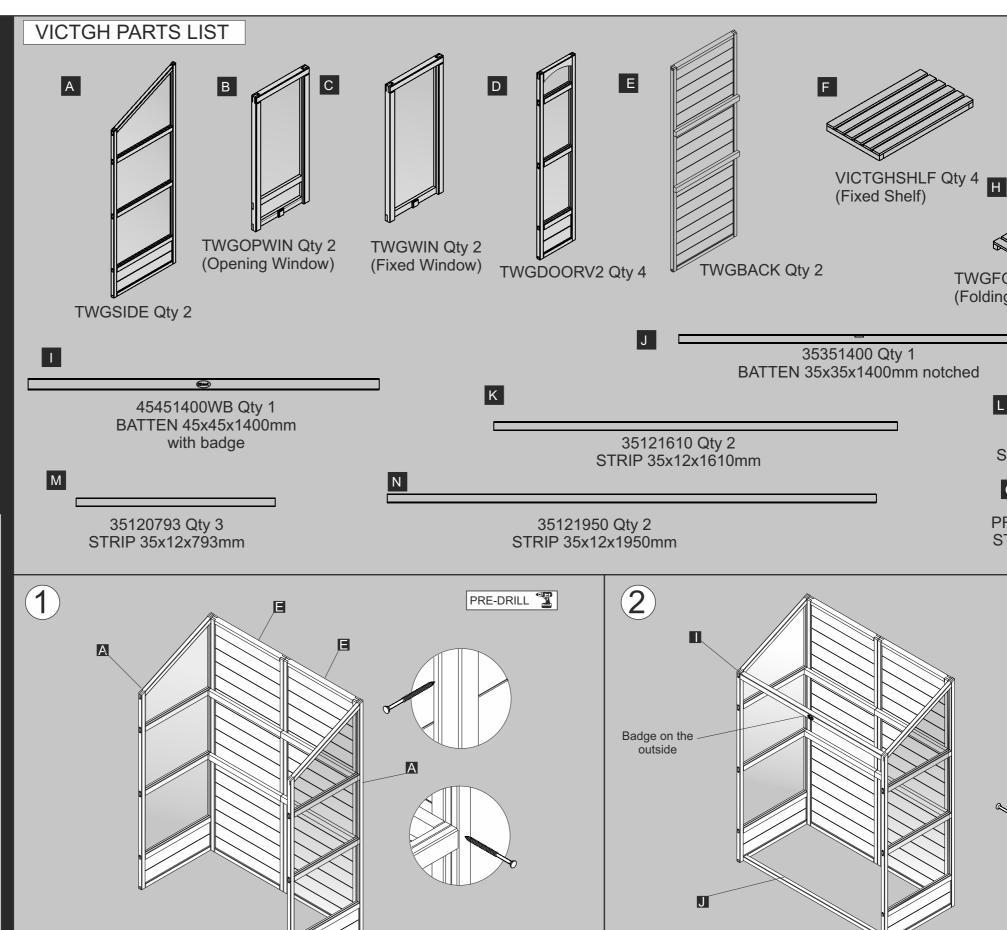
Fix the side panels to each of the back sections, screwing through the outside of the side panels into the back panel, using 3 x 60mm screws for each.
