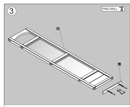
Fix a 347mm strip to the bottom of two of the doors using 2x30mm screws for each.
