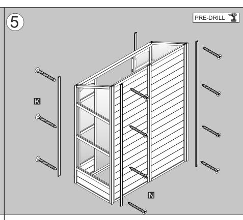
Fix the cover strips to the front and back of each side panel making sure that each is flush. Fix these in place using 30mm screws.
