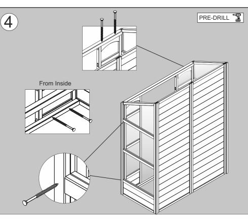
Place the two sections that you have just completed in step 3 against the front of the green house. Fix each in place doing the following.
