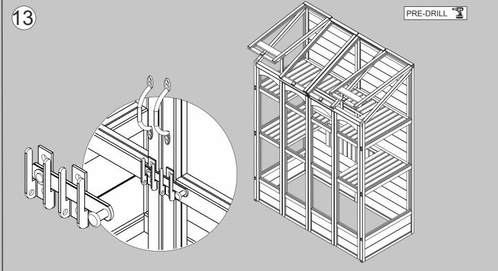
Fix a handle to each of the doors making sure that these are in line with each other. Fix each in place using 25mm screws.
