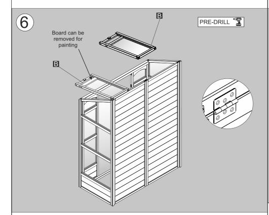
Fix two hinges to the back of each opening window using 3x25mm screws for each hinge. Place the windows on top of the frame making sure that they are square and in line with the side panels and fix the other half of the hinges to the back panel using another 3x25mm screws
