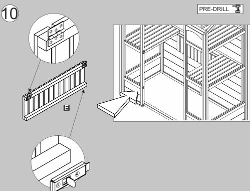
Fix two hinges to the underside of each (folding shelf) using 3x25mm screws for each hinge. Fix a bolt to each end of the opposite batten using the screws provided.
