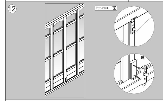
Close the left hand door which you have just fixed. Place the LOCKBLOCK on the inside of the door so that it is in line with the framework and sits at least 3mm above the bottom batten. Fix the block in place using 2x30mm screws.
