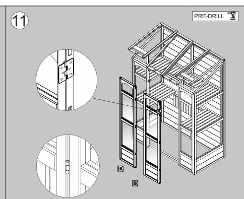
Fix two hinges to the side of each TWGDR as shown using 3x25mm screws for each hinge. Place these against the panels you previously fixed in step 4 so that the hinge is against the inside of the frame and secure the other half of each hinge using 3x25mm screws.
