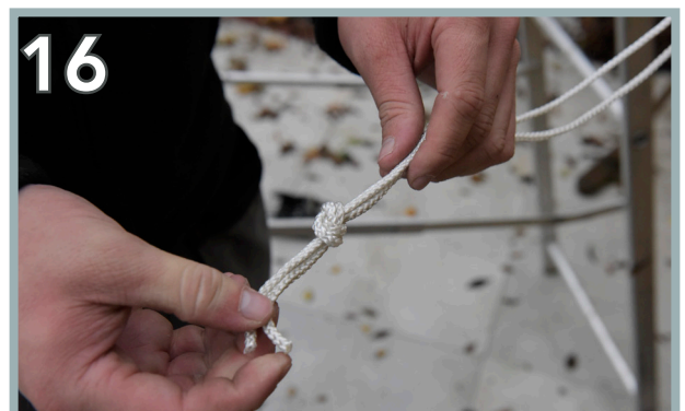
Using the two ends of the ropes that have been threaded through the Large Roller, tie them in a knot as shown above.
