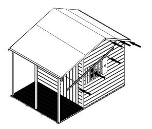
Place the **40100850A1CRCTPTR** and the **40101384ACRCTPTR** against the sides of the building so that each is flush withe the top of the roof and they meet up to one another at the apex.
