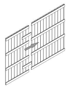
Slot the two floor section (RP02FL and RP02SFL) together on the floor. Make sure that the smaller section is towards the back of the building. Do not fix together.
