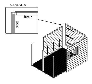
Place the **RP02SP** onto the **RP02FL** as shown so that it is flush with the outside and the back.
