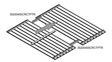
Fit the **RP02SR** to one of the **RP02LR** sections as shown.
