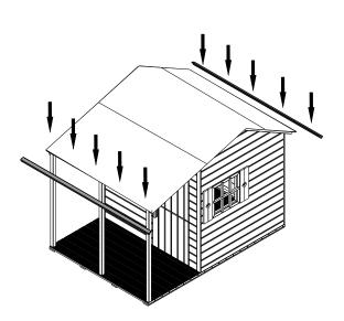
Fix the two **35201500SCRCTPTR** to the overhang of the **RP02LR** and the **RP02SR** so that it overlaps the felt. Secure each in place using 5x13mm screws.
