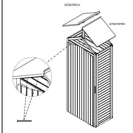
Position the door end against the building and secure this in position as you did the back end, using  $3 \times 60$ mm screws, evenly spaced, screwing through the door end into the side panels.
