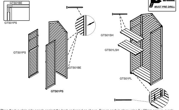
Place the two plain side panels against the back end panel as shown. Secure each in place using  $3 \times 60 \text{mm}$  screws, evenly spaced, screwing through the end panel into the sides.
