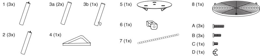
Prior to assembly, read the instructions carefully. Check all parts against this parts list. Carry out assembly on a soft surface to avoid scratching the paint. Please retain this information for future reference.
