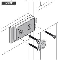
Attach the Door Handle and Escutcheon to the external face of the 'opening' Door using their supplied fixings.
