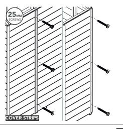
Attach the Joiner Cover Strips to the Apex Sections. Ensure they are flush to the Cover Strips.
