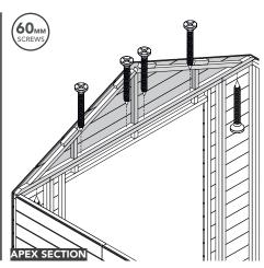
Attach the back Apex Section to the back panels and attach the Internal Apex Section to the Internal Panels as shown below.
