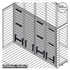
Attach the front Apex Section screwing to the front panels as shown below.
