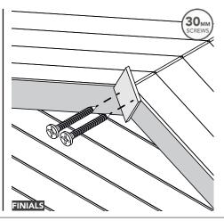
Secure the Finials with screws to the attached
