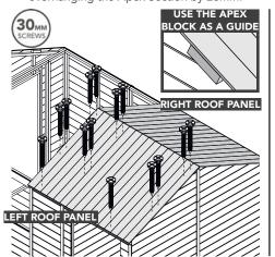
Secure the front Roof Panels to the battens attached to the Apex Section, and Truss. Ensure the front Roof Panels are butt up against the back Roof Panels.
