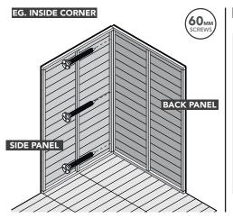
Repeat the process for the remaining panels and **secure** the **panels together**. Make sure that the bottom frame of the wall panel rests on the outer edge of the floor.
