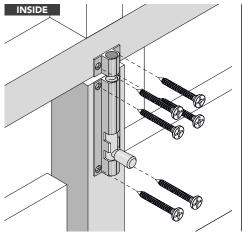
Fix a Barrel Bolt to the top of the Slamming
