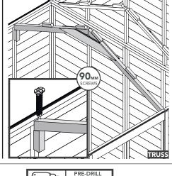
Secure the back Roof Panels to the battens attached to the Apex Section, Internal Apex Section and Truss. Ensure the Roof Panels are overhanging the Apex Section by 28mm.
