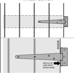
Position and **attach the hinges** to the framework behind on the Door. **Please take** note of the hinge position.
