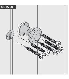
Position and secure the Rim Lock Receiver to the Slamming Strip. Test the key to ensure the lock works accordingly.
