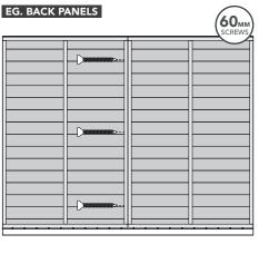
Secure the panels into place by screwing into the floor bearers.
