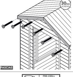
Secure the Fascias with screws to the attached
