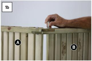
Interlock joints in Seat Back (A) with Seat (B) as shown in Fig. 1 and secure using 6x 45mm bolts, nuts & washers. (2x 45mm bolts per joint).
