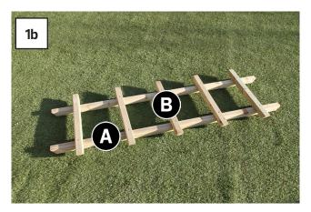
Position Rafters B at both ends of Rails A and fix using 4no 60mm Screws – 2no per Rafter (Fig.1a). Space out remaining Rafters B evenly (Fig.1b) and attach using 6no 60mm Screws.
