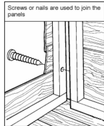
The wall panels are secured to the floor joists using 60mm screws. If nails, knock them in at an angle (skew nailing).
