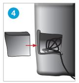
Place the pump and excess wires into the access cavity ensuring that the long pump/L.E.D. wires extend out through the opening. Cover the opening with the trap door.
