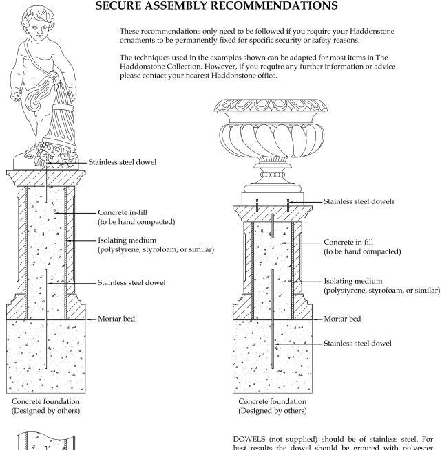
It is essential that the base stone is levelled on a continuous mortar bed Foundations designed by others to suit site conditions and loadings ALTERNATIVE
