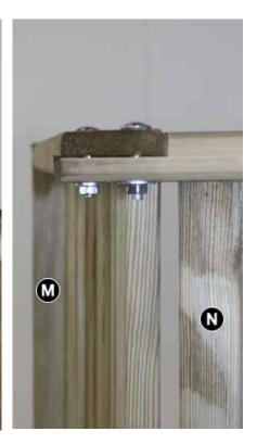
Interlock joints in Seat Back (M) and Seat (N), align bolt holes and secure using  $6 \times 45$ mm Bolts, Nuts & Washers. (2 x Bolts per joint) do not tighten fully at this stage.
