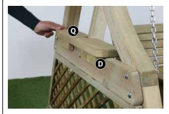
Place Shelves (Q) on to Horizontal Short Braces (D). Tap in with a mallet to fit.
