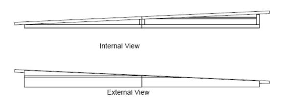
Note - Please ensure that the 4ft pent top is on top of the 4ft panel and any 2ft pent tops are placed up on the 2ft panels as this will ensure that the cover lats align.
