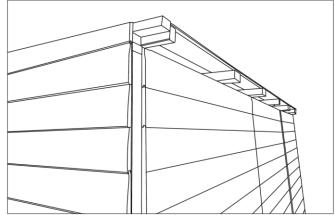
If the framing does not align the base may be very slightly out and the two opposite corners of the floor may need lifting. More details on bases can be found on www.powersheds.com/how-to-build-a-shed-base/
