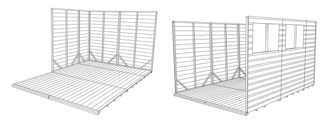
9. When you have secured all the wall panels (door panel, 2ft and 4ft blank panels, window panels) you then need to secure these to the floor using 70mm screws provided. Screw into the floor with 2x screws for every wall panel (internally) ensuring the screws are driven through the framing at the bottom of the side/gable walls, through the floor boards and into the floor joists.
