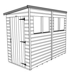
2. Secure corner strips at each corner of your Power shed with 40mm nails (at least four per strip). Extra strips are provided to cover any joins between side wall panels.
