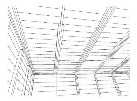
**Note** – The roof panels are not handed, it does not matter which way round they go.
