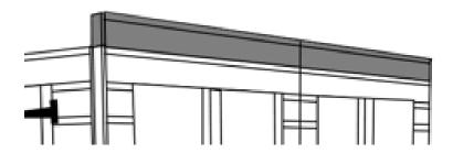
2. Line up the gable tops with the panels at the gable ends (the ends where you attached the 'heavy duty bearers') and secure them to the wall panels with 50mm screws from the inside, screwing upwards through the framing. The gable tops will come in two halves.
