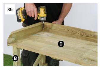
Place Worktop Assembly (D) onto the framework ensuring open edge of Worktop Assembly is flush with front face of side frames and screw down into legs using 4x 50mm screws (1x 50mm screw per corner) (See Figs 3a & 3b).
