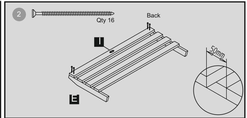
Place the long battens across the shorter battens to create the bench seat and back. Make sure that the battens for the bench are spaced 50mm apart. Fix each in place using 2x60mm screws for each end.
