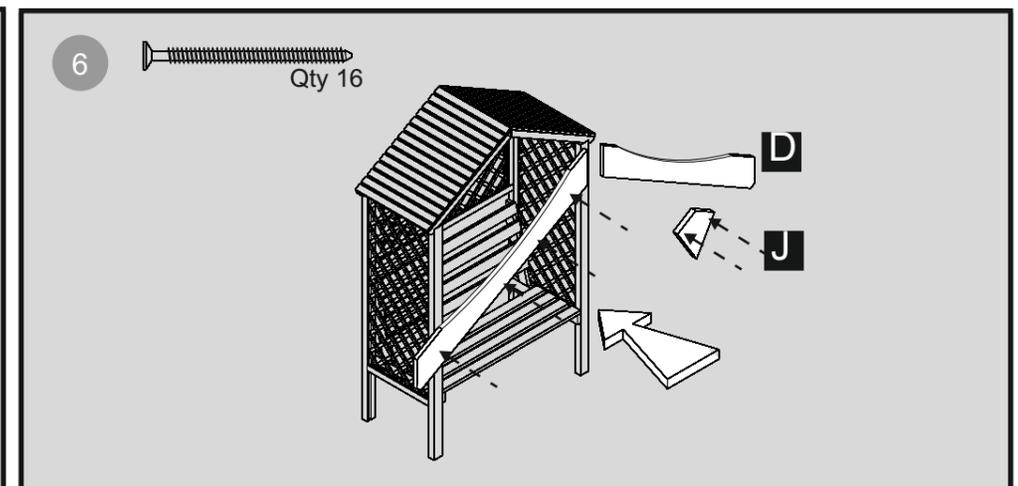
Place the barge boards to the roof so that the bottom of the curve is in line with the top of the roof and they meet at the apex. Fix each in place using 3x40mm screws, Place the finial over where the barge boards meet and secure each in place using 2x40mm screws.
