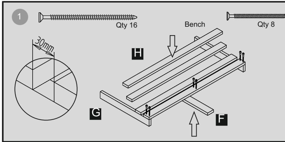
Make sure that the battens for the bench are spaced 30mm apart. Fix each in place using 2x60mm screws for each end.
