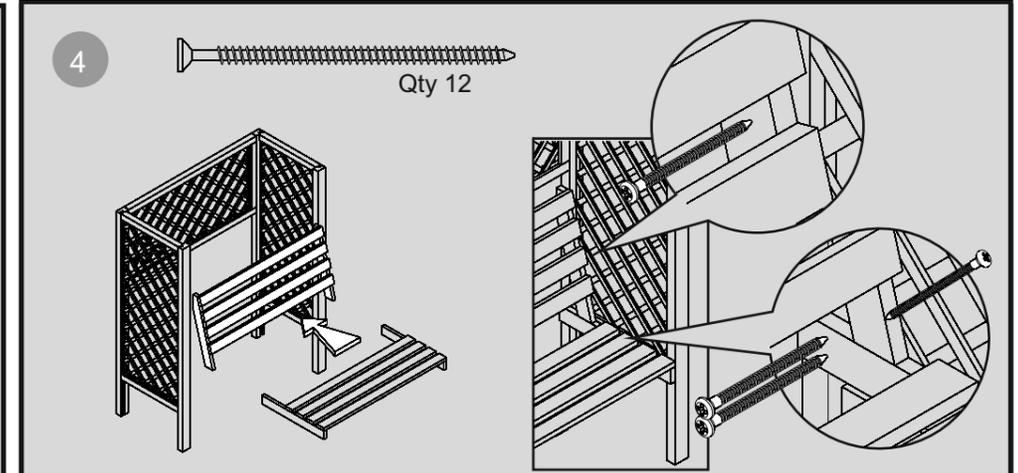
Place the bench seat between the two sides so that it is tight and the bottom of the bench is 378mm from the ground. Fix this in place using 2x60mm screws to fix each end to the posts of the sides sections .
