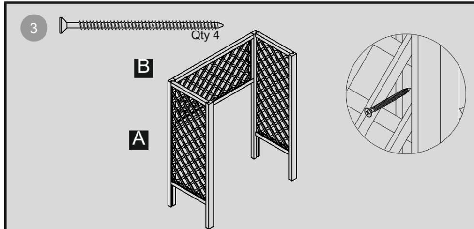
Fix the back panel to both of the side panels making sure that it is in line with the top. Fix this in place using 2 x 60mm screws for each side screwing through the groove in the panel.
