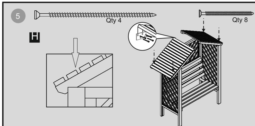
Fix the two roof sections together and secure using the metal plates and 8x40mm screws as shown.
