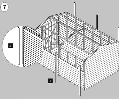
Place the 1710mm strips so that they cover the joins at each corner and between the panels. Fix each corner strip in place using 3x30mm screws and each middle strip with 3 x 40mm screws
