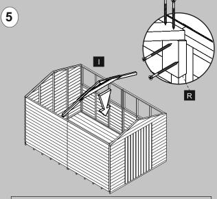
Place and secure each angled block using 2x70mm screws. Make sure these are 1470mm from the floor level and are tight against the framework.
