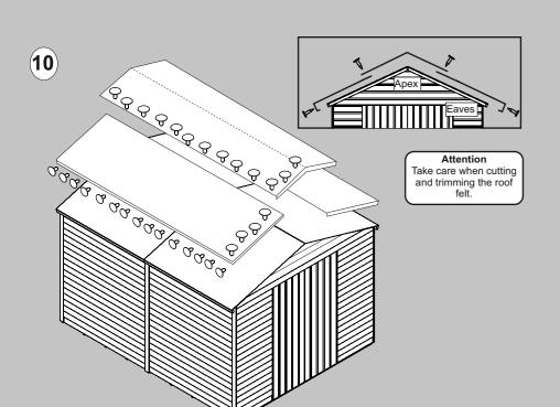
Unroll the felt and place a section on to each eaves so that there is a 50mm overhang on the three edges as shown. Fix this to the roof using felt nails spaced in 150mm intervals. Cut and fold the corners securing with a single felt nail for each.
