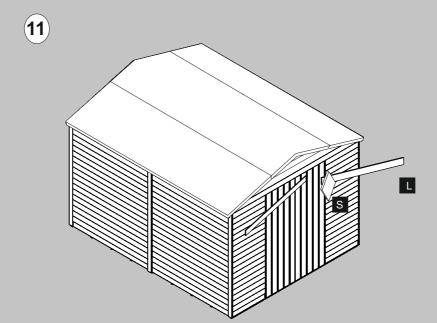
Place the barge boards against the front and back of the shed. Make sure that these are in line with the roof sheet and meet at the apex. Fix each in place using 3 x 40mm screws.
