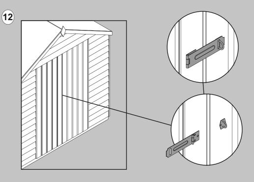
Before fixing the Hasp to the door, make sure that it is in line with the framing on the reverse of the door and that it closes over the Staple. Fix this in place using 3 x 25mm screws.
