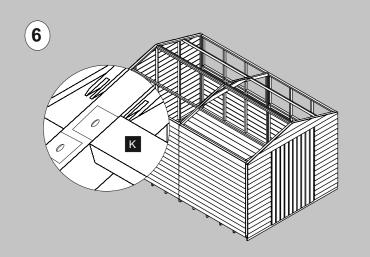
Secure a Z' bracket to each end of the 1757mm battens using a single 25mm screw for each bracket. Position the battens as shown so that there is four battens on either side of the truss and the Z' bracket sits on the framework. Secure the battens in position using a 25mm screw for each Z' bracket.
