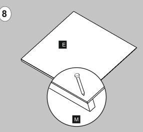
Place a roof sheet on top of one of the 1835mm battens. Make sure the board is sat on the narrow side of the batten and that it is flush on all sides. Fix this in place using 30mm nails spaced at 300mm intervals.
