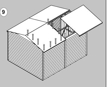
Lift each roof sections into place making sure that they are in line with the apex. Ensure that it is flush with the front and back panels of the workshop.
