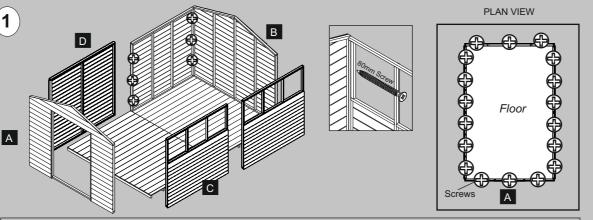
Place the panels on top of the completed floor. Make sure that all the panels are tight and flush before fixing them to each other using 3x50mm screws
