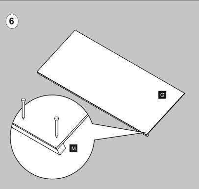
Place the roof board on to one of the 1791mm battens. Make sure that the board is flush on all sides.
