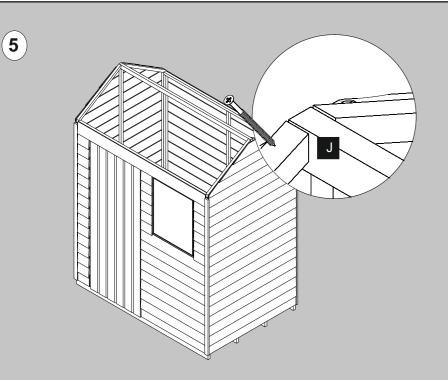
Place the 1753mm batten so that it connects the door end and plain end. Fix this in position using a 50mm screw for each end as shown.
