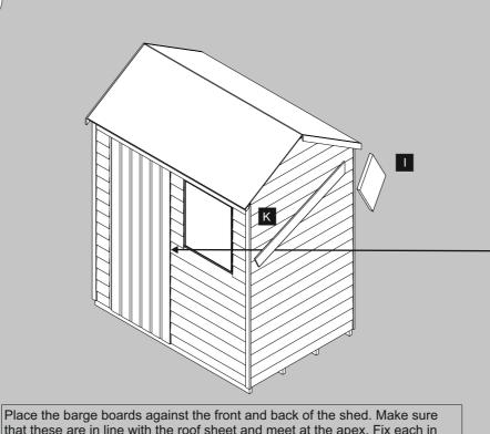
that these are in line with the roof sheet and meet at the apex. Fix each in place using 3 x 40mm screws.
