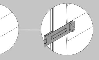
Position the staple on the door end in line with the centre batten on the reverse of the door. Making sure that the staple is in line with the framing behind, fix it in place using 2 x 25mm
