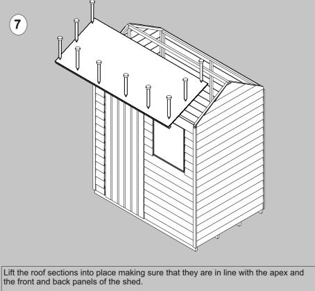
Fix the roof in place using 30mm nails spaced in approximately 300mm intervals. (Make sure the nails locate into the framework of the panels)
