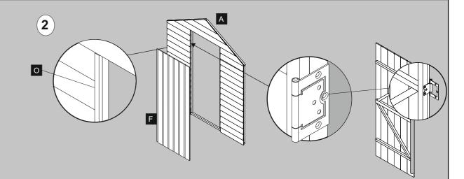
Fix the 20 x 1695mm strip to the side of the door frame so that it is tight with the cladding and flush with the frame. Use 3 x 30mm screws.
