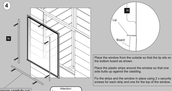
the bottom board as shown Place the plastic strips around the window so that one
