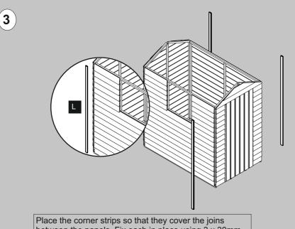
between the panels. Fix each in place using 3 x 30mm screws
