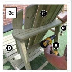
Position Armrest/Leg Assembly D1 as shown in Fig 3a. Align bolt holes and insert 2x Hex Bolts and 'T' Nuts. See Fig 3b. Do not fully tighten.
