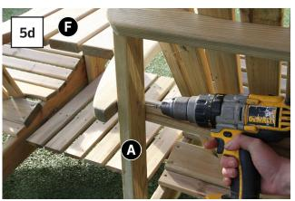
Place shelf assembly between seat assemblies (D1 & D2 outermost) Fig 5a, locate screw/ bolt holes and attach using 4x Hex Bolts & 'T' Nuts to front (Fig 5b) and 2x Hex Screws to rear (Fig 5c).
