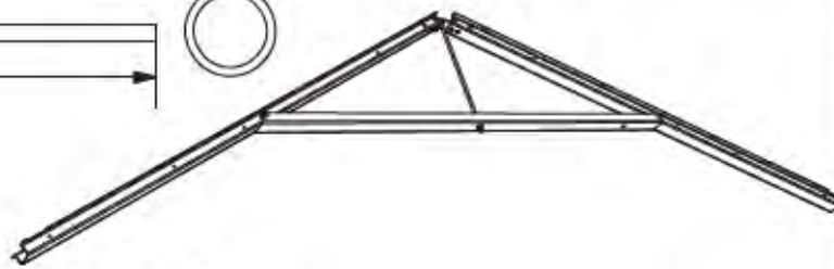
Truss Assembly (x2)
