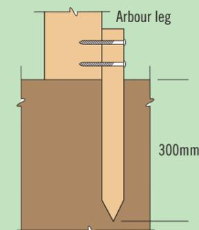
Arches have longer legs and should be embedded into soft ground. Fix the legs in place using a post-fix product such as MetCrete.
