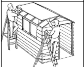
On the inside of your building there are roof spars that meet in the middle, fix these together using the triangle shaped roof ties using 4no. 40mm lath nails. This will help secure the roof and stop it from sagging.
