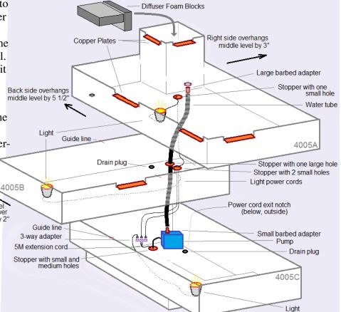
4) Thread the smaller barbed adapter into the top of the pump. Press one end of the water tube onto the adapter.
