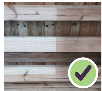
Sun Bleaching & Green Spotting are not causes for concern and they will fade over time when items are placed outdoors.
