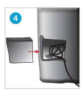
Place the pump and excess wires into the access cavity ensuring that the long pump/L.E.D. wires extend out through the opening. Cover the opening with the trap door.
