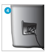
Place the pump and excess wires into the access cavity ensuring that the long pump wires extend out through the opening.
