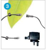
Connect the two ends of the L.E.D. lighting wires together and screw over the plastic collar. Push the cable with two pins into the transformer plug and screw over the plastic collar.
