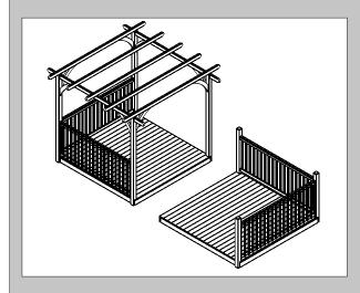
Fix the two decks together at step 3 screwing the deck boards together.
