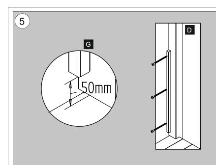
Place a baluster against the post so that it is 50mm above the deck and flush with the outside of the post. Fix this in place using 3 x 50mm screws. Repeat for the other posts.
