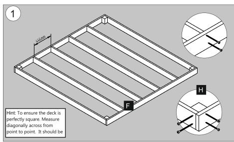
Use four of the boards to create your square base as shown. Fix at the corners using the blocks provided.
