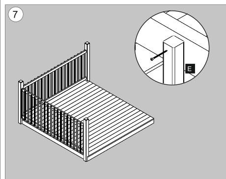
Fix the remaining balusters to the outside of the rails making sure each is spaced approximately 91mm apart.
