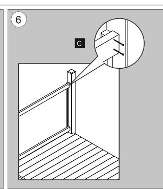
Measure the distance between the posts and cut the rails to the correct size so that they can fit in between the posts.
