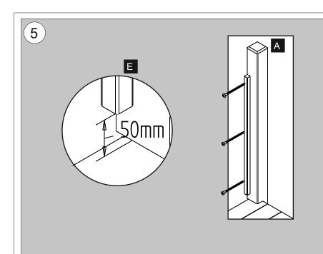
Place a baluster against the post so that it is 50mm above the deck and flush with the outside of the post. Fix this in place using 3 screws. Repeat for the other posts.
