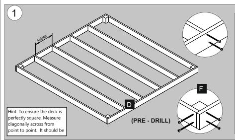
Use four of the deck boards to create your square base as shown. Fix at the corners using the blocks provided and 2 x 50mm screws at each end of each board.
