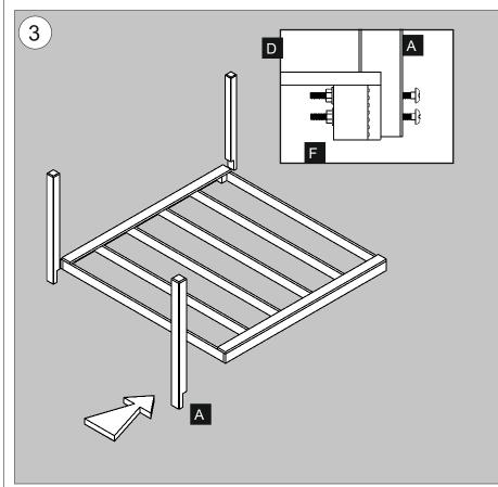
Place a post against the corner so that the notch sits on the deck board you have previously placed. Make sure this is tight and flush.
