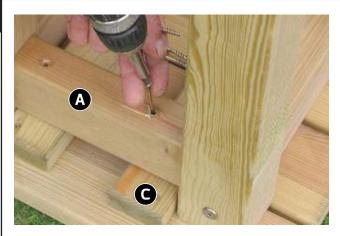
Place Legs/Braces Assembly onto Table Top C and fix in position using 4  $\times$  120mm Screws.
