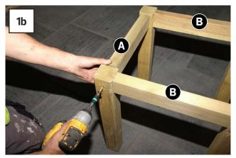
Attach Braces A to Legs Assembly B using  $4 \times 110 \text{mm}$  Hex Screws (2 per Brace) as shown.
