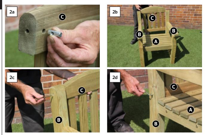
Insert 4no Cross Dowels into 10 mm holes to rear of Back Assembly (C) ensuring slots face outwards (Fig. 2a). Position the Back Assembly between side assemblies (Fig. 2b) and insert 2no bolts per side and thread bolts into cross dowels (Figs.2c & 2d).
