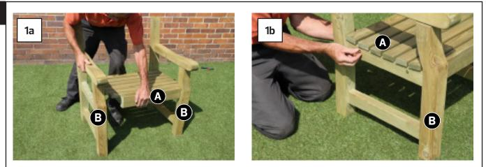
Position Seat Assembly A between Side Assemblies B (Fig.1a). Align bolt holes and attach using 4no 105mm Bolts, Washers and Nuts (Fig.1b).
