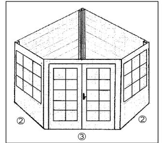
Slide roof onto the building. Starting in back corner, ensuring there is approx a 25mm overhang, screw roof from inside up through rail into the roof. Make sure the roof is squared up to the building and there is a 25mm overhang all the way round. Once this is done secure the roof in the same way as before.
