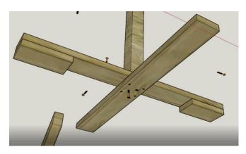
3. Position the 4 x angled supports onto the base, ensuing that they are flush to both the base and the post. Fix each each support using 2 x 50mm screws, one through the base and one through the post in each support.
