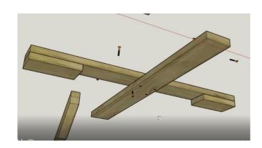
Position the bird table post onto the centre of the base and screw together through the underside of the base using 2 x 100mm screws
