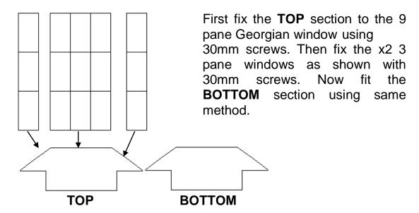
Finally glaze all the windows from the inside, and fix securely with the window latts provided. Once done run a line of silicone sealant (not supplied) around each window on the outside to stop any leaks from occurring.
