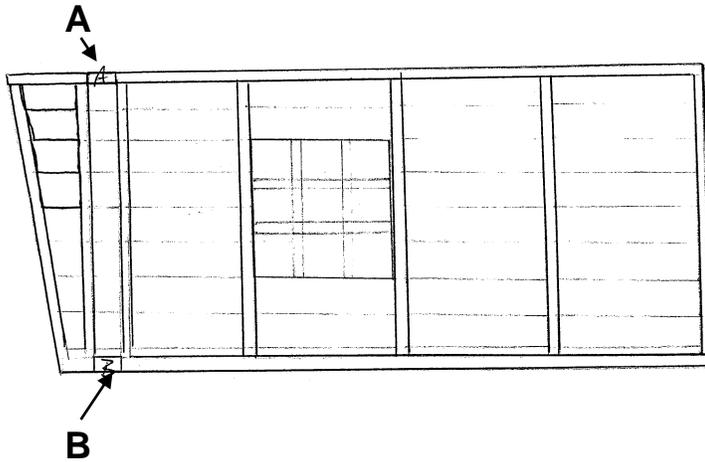
The panels are joined to each other through pre-drilled holes, using 80mm coach screws. It is usual to start with a side and back panel, then to add the other side panel. The action of tightening the screws draws the wall panels together.
