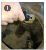
Feed the pump plug and cable through the PVC pipe in the base of the water reservoir and pull it out through the notch underneath.
