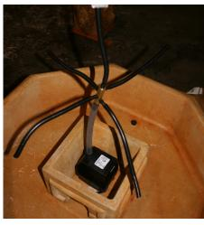
Put the small pedestal in the centre of and attach the thin black tubing over each of the black nozzles, push the wider nozzle into the open end of the clear tubing ensuring that the longest length of black tubing is on the top of the manifold, slide the metal clamp over the long black tubing and tighten just enough to hold in place.
