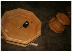
STAGE 3 Sit the large hexagonal bowl on two wooden batons (found Inside the box) and feed the pump cable through the central hole and then through the top of the large pedestal and out through the bottom. There is a notch in the bottom of the pedestal for the cable to run through; this notch should be at the closest point to the power source.
