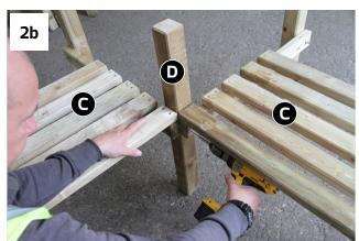
Attach 2x Notched Posts A and 1x Full Post B to remaining seat C (ensuring notches facing outwards) using 3x Bolts, Washers & Nuts –1x per post. See Fig.2a. Attach seat and posts assembly to Table Leg D using 2x 60mm Screws -Fig.2b
