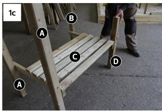
Attach 2x Notched Posts A and 1x Full Post B to seat C (ensure notches face outwards) using 3x Bolts, Washers & Nuts –1x per post. See Fig.1a & 1b.
