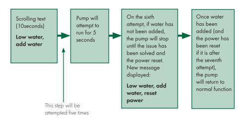
**IMPORTANT:** when the power is being reset, turn the pump off at the mains power supply for a minimum of 5 seconds - this will allow the components of the controller to fully reset.
