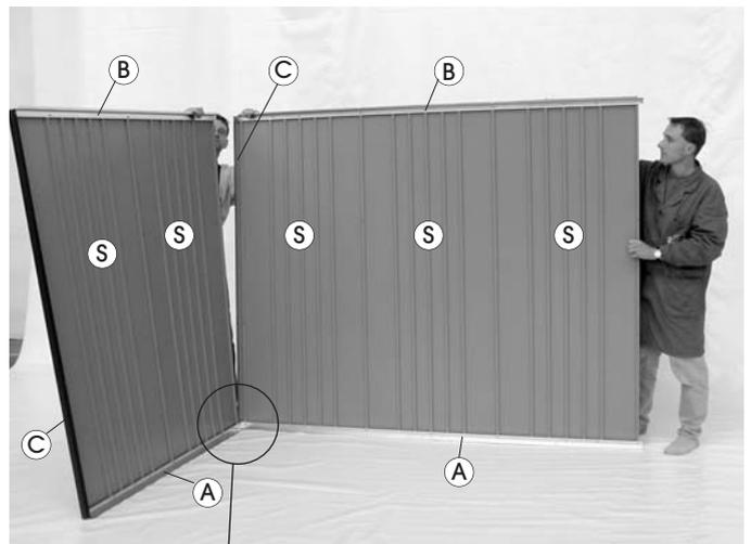
**GB** Now assemble the back and the side wall elements together. Do not connect the ends of the top frames **B** together with bolts just yet (see arrow). Finally attach the front wall element and adjust all the walls to be at right angles to one another. For the sizes 2A – 7 mount the brackets for the door hooks on the upper left and right corners of the front wall. The top and bottom frames of the front and back walls should overlap the profiles of the side walls (see detail)
