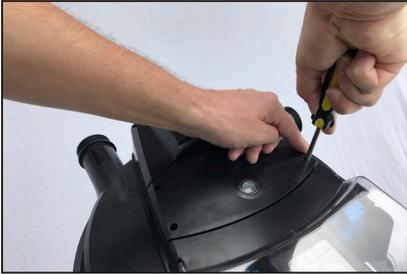
**Step 1** - Unscrew the four screws under the rubber plugs on the lid of the UV-unit.
