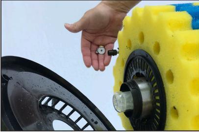
**Step 5** - Please take care not to lose the plastic bearing on the foam side of the plate when removing the base plate.
