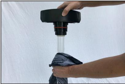
**Step 3** - Clean the quartz glass tube with a wet cloth and dry.
