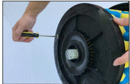
**Step 4** - Using a screwdriver (not supplied) - unscrew and remove the washer and screw.
