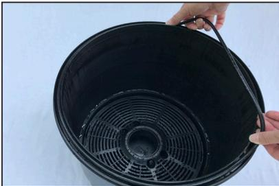
**Step 8** - Fit the O-ring in place on the top of the cannister (to facilitate the placement of the lid, you can use silicone grease (preferred) or make the O-ring wet. The lid can then be pressed in place and the large clamp be mounted from the hinge side and locked.
