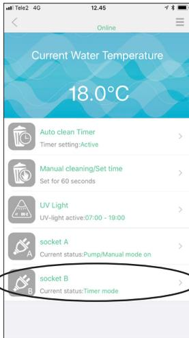
28. Socket B can be used for all pond-equipment like feeder, dosage pump, light etc. Max. 800W total on both A+B
