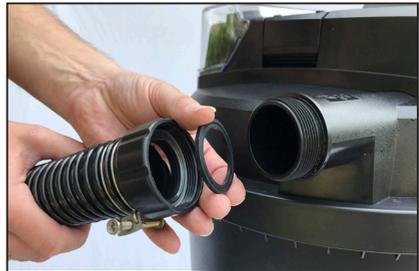
**Step 9** - Now refit all the hoses again – remember to insert the flat gaskets and tighten the locking nuts.
