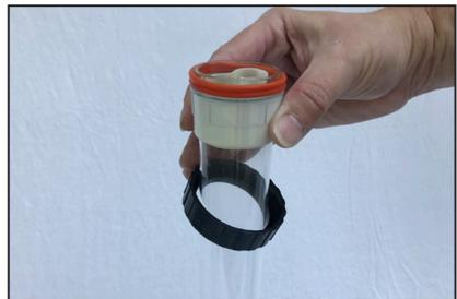
**Step 6** - Check the quartz glass tube and change it if broken. Ensure all o-rings are in place and greased with silicone grease.
