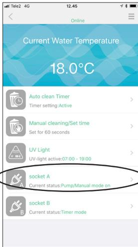
25. Socket A is reserved for the pump supplying the filter ! Assuring safety and functions. Max. 800W total on both A+B
