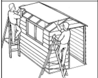
On the inside of your buildings there are roof spars that meet in the middle, fix these together using the triangle shaped roof ties using 4no. 40mm lath nails. This will help secure the roof and stop it from sagging.
