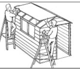
On the inside of your buildings there are roof spars that meet in the middle, fix these together using the triangle shaped roof ties using 4no. 40mm latt nails. This will help secure the roof and stop it from sagging.
