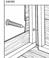
The panels are joined to each other through predrilled holes, using 80mm coach screws. It is usual to start with a side and back panel, then to add the other side panel, and finish with the door section. The action of tightening the screws draws the wall panels together. Subsequent panels are secured to each other.
