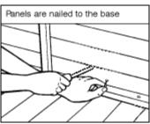
The wall panels are secured to the floor joists using 60mm screws. If nails, knock them in at an angle (skew nailing).
