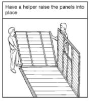
The panels are joined to each other through predrilled holes, using 80mm coach screws. It is usual to start with a side and back panel, then to add the other side panel, and finish with the door section. The action of tightening the screws draws the wall panels together. Subsequent panels are secured to each other.
