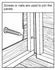
The wall panels are secured to the floor joists using 60mm screws. If nails, knock them in at an angle (skew nailing).
