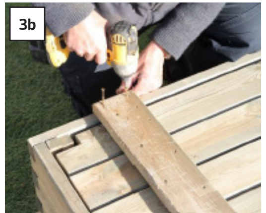
Invert the planter and place the base as shown in Fig.3a. Fix in position using 12no 70mm Screws – 2no per bearer (Fig.3b)
