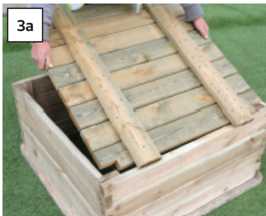
Invert the planter and place the base as shown in Fig.3a. Fix in position using 8no 70mm Screws – 2no per bearer (Fig.3b).
