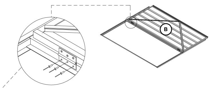
NOTE: NUTS AND BOLTS (SUPPLIED) MAY BE USED INSTEAD OF POP RIVETS (SUPPLIED) BY SIMPLY ENLARGING THE HINGE HOLE SETS IN THE JAMB USING A 4MM DRILL BIT
