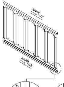
To pre-assemble the four wall panels and two roof panels, the perimeter channels are secured to the top and bottom of each panel using the snaptite system, as detailed on the following pages wherever you see the symbol.  $_{\rm SNAP}$
