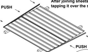
Position sheets on timbers, trestles or partly over edge of concrete slab.
