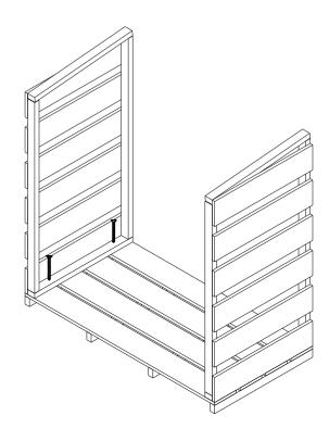
Place the left hand side on to the floor short side as shown and secure using 2x50mm screws, screwing into the batten underneath.
