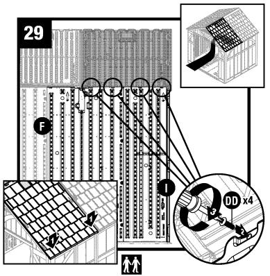
Pull down each lower corner of roof from outside. From inside shed, attach tabs on right front corner (I) and side panel (F) to roof panel with four screws (DD).
