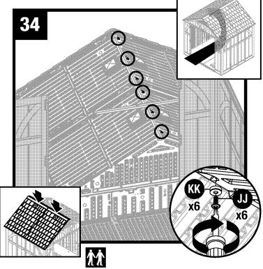
Push down the roof from outside. From inside shed, secure roof panels together along ridge of roof using six rubber washers (KK) and six sealing screws (JJ).
