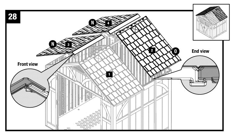
Repeat Steps 25-27 for remaining roof panels. Install panels in the order shown.
