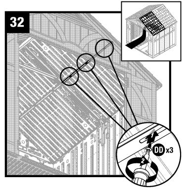
Secure roof support to roof using three screws (DD).
