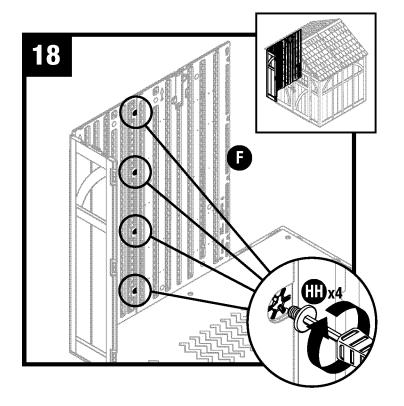
Secure side panel (F) with four easy bolts (HH), working from floor to roof. **DO NOT** use torque wrench. Use easy bolt easy driver (II) and hand tighten. Easy bolt head will be flush when fully seated. **DO NOT** over tighten easy bolts.
