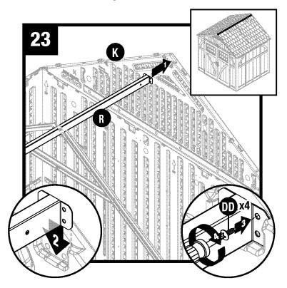
Raise ridge beam (R) up and into rear header (K). Secure with four screws (DD).
