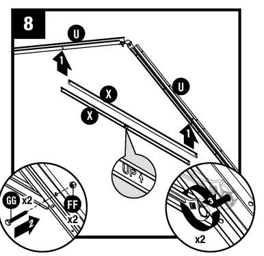
Attach two truss cross beams (X) to two truss legs (U) with two hex bolts (GG) and two nuts (FF). Stand truss and check cross beam is level.
