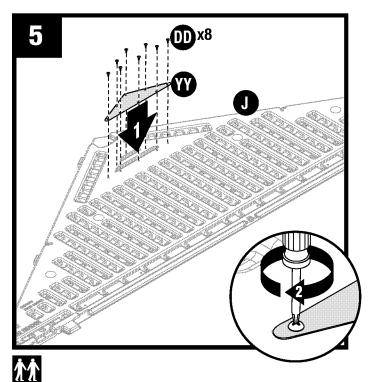
Lay front header (J) on ground with lettering side facing up. Place fiberglass vent screen (S) into rear opening in front header (J). Secure with eight screws (DD). **DO NOT** over tighten screws.
