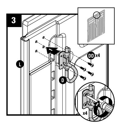
At top interior side of left door (L), attach D-ring slide bolt (D) with four screws (DD).
