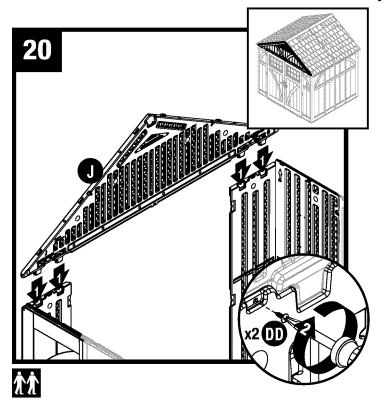
Place front header (J) over door opening and fit four protruding support legs into pockets molded in front corners. Secure front header using two screws (DD).
