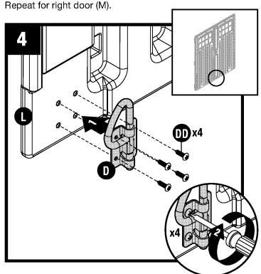
At bottom interior side of left door (L), attach D-ring slide bolt (D) with four screws (DD).
