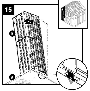
Tip left front corner (E) back to vertical position and align lower tabs on right side with slots in floor (A).
