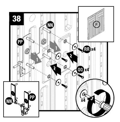
Insert screw stems, on left and right handle plates (NN) and (PP), through the pre-drilled holes in doors. While holding plates in place on exterior of door, secure each with two washers (QQ) and two machine screws (RR).
