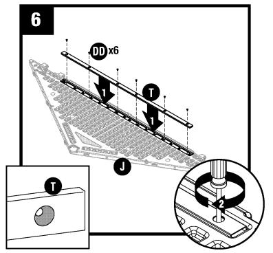
Place header beam (T) into pocket of front header (J). Secure with six screws (DD). **DO NOT** over tighten screws.
