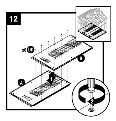
Push left floor (A) and right floor (B) panels together and secure with six screws (DD).
