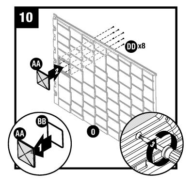
Place skylight gasket (BB) into skylight (AA). Place skylight (AA) onto right roof panel (O). Secure from underside with eight screws (DD). Make sure rib on plastic parts is seated fully against gasket on skylight.
