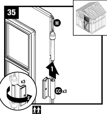
Stand right door (M) upright with three hinge mounts facing right. Slide one metal door hinge (CC) up onto each hinge mount. Rotate door hinges to outside of door.
