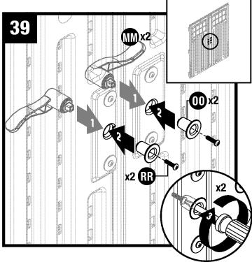
From the outside of doors, insert door handles (MM) through handle plate holes. On inside of doors, place spacers (OO) on each door handle, and secure each with one machine screw (RR).
