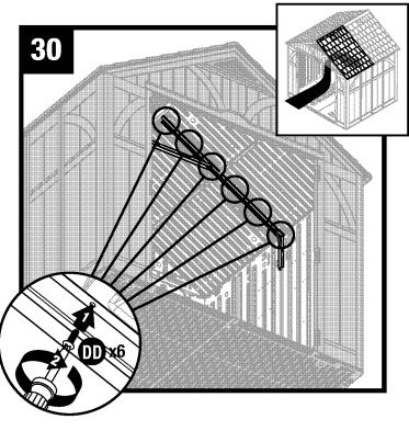
Secure roof to truss using six screws (DD). Each screw will attach at a corresponding screw boss on the roof.
