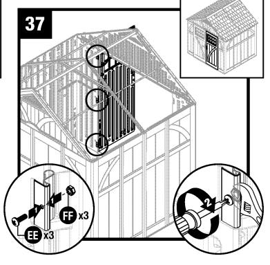
Secure each metal hinge plate with one screw (EE) and one nut (FF).
