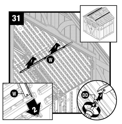
Raise roof support (W) into position against roof. Slide roof support (W) into front header. Secure roof support (W) to underside of truss leg with one screw (DD).
