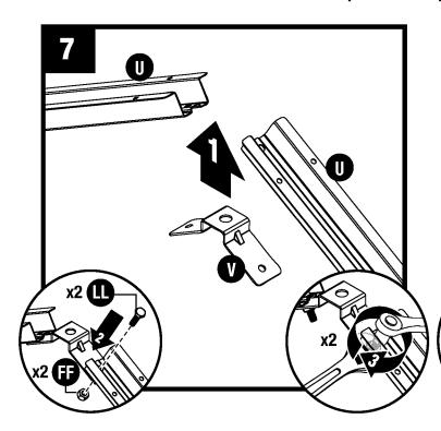
Attach truss bracket (V) to end of one truss leg (U) with one hex bolt (LL) and one nut (FF).
