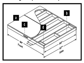
Secure shed to wood platform using 1/4" x 2" lag screws.
