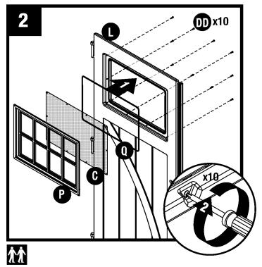
Place gasket (Q), window (C), and frame (P) into door channel. Secure with ten screws (DD), starting at corners. **DO NOT** over tighten screws.
