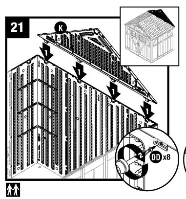
Place rear header (K) over back walls and fit four protruding support legs into pockets molded in back walls. Secure rear header using eight screws (DD).
