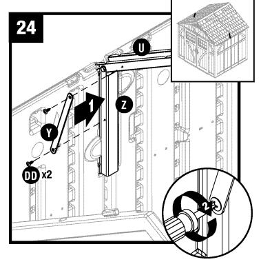
Attach truss strap (Y) to side adaptor bracket (Z) and truss leg (U) with two screws (DD).
