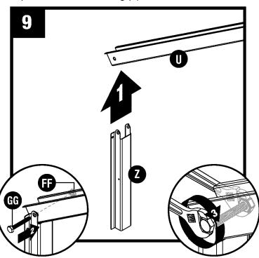
Attach side adaptor bracket (Z) at end of left truss leg (U) with one hex bolt (GG) and one nut (FF).
