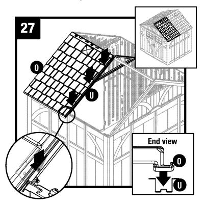
Press edge of right roof (O) into channel on truss leg (U).
