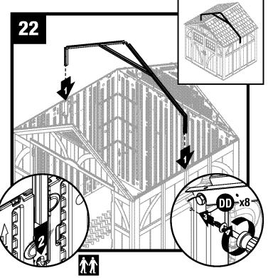
Slide truss assembly into place. Secure with four screws (DD) in each side adaptor bracket.
