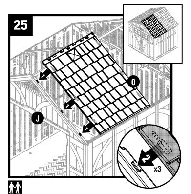
Lay right roof (O) directly over three tabs on right side of front header (J). With right roof slots seated over/on header tabs, check alignment in all three spots.
